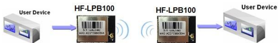
Figure 34. 透明串口应用图示
